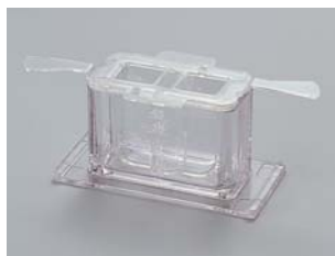
Small sample cup (10ml) Used when measuring small volume samples
