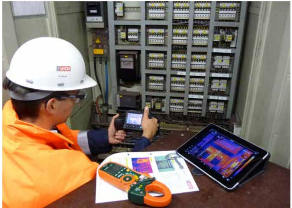
Michael Weigt performing thermography: the data from the Extech clamp meter are transferred to the thermal imaging camera via Bluetooth. The FLIR T440 transfers the thermal images to a tablet PC via Wireless LAN.
