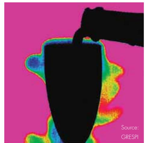
*Researchers used a FLIR SC7000 series thermal imaging camera to visualize CO<sub>2</sub> as it escapes during the pouring of a glass of champagne.*
