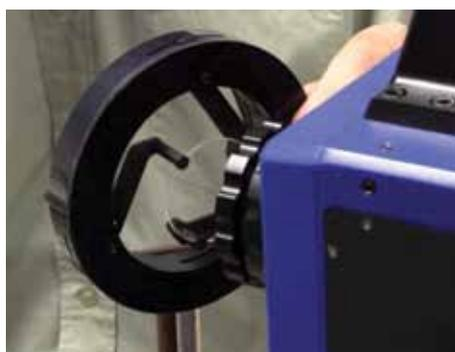
To visualize the escaping CO<sub>2</sub> the researchers used an external band-pass filter.
