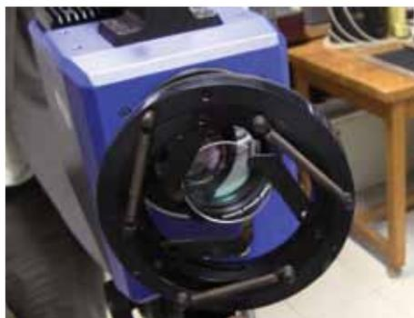
The external band-pass filter is centered on the CO<sub>2</sub> emission peak.
