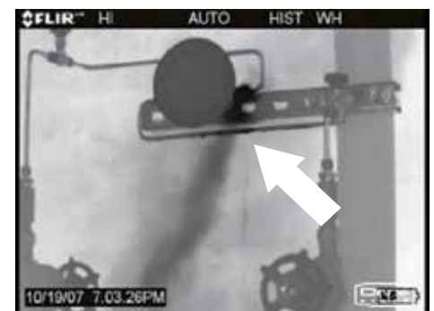
A leaking pressure gauge
