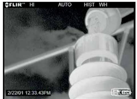
*During their first FLIR training course, SSEPD identified a leak on a recently installed high-voltage circuit breaker.*
