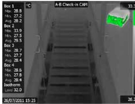
*Suitcases do not trigger the alarm, even if the threshold temperature is reached. The percentage of the ROI that reaches that temperature is too small.*
