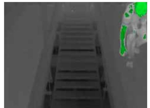
Field tests have shown that if a person enters the conveyor belt area the automatic temperature alarm will immediately stop the conveyor belt system.
